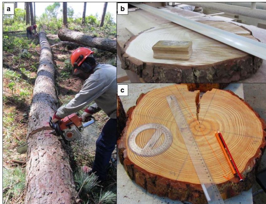
FIGURE 4.2-1: (A) CROSS-SECTIONAL DISCS SAMPLING; (B) BAND SANDING MACHINE AND (C) DISC READY FOR DIGITALIZATION.
