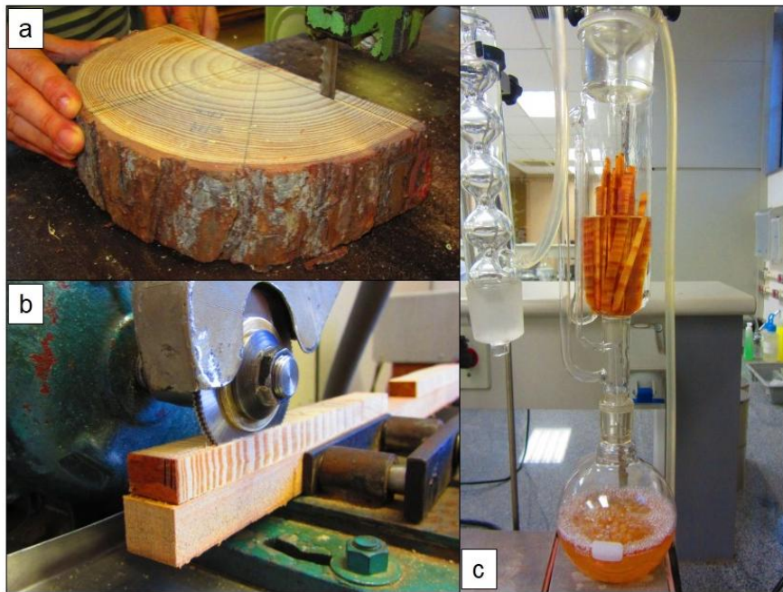
FIGURE 5.2-1: (a) WOOD SAMPLE FROM THE CROSS-SECTIONAL DISCS AND (b) THROUGH TWIN-BLADED CIRCULAR SAW. (c) SOXHLET APPARATUS USED ON THE RESIN EXTRACTION
