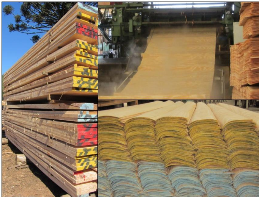
FIGURE 7.1-1: PRODUCTS OBTAINED FROM THE EVALUATED INDUSTRIAL PROCESSES. SAWTIMBER OF DIFFERENT DIMENSIONS (LEFT); ROTARY PEELED VENEER TOTALLY FREE OF DEFECTS (UP RIGHT); AND SLICED VENEER SHEETS (DOWN RIGHT)
