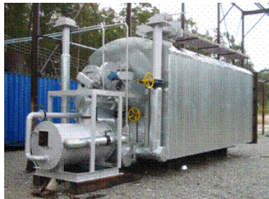
Figura 4.9. Processo DPC ( Drying Pyrolysis Cooling ) (SANTOS, 2007).
