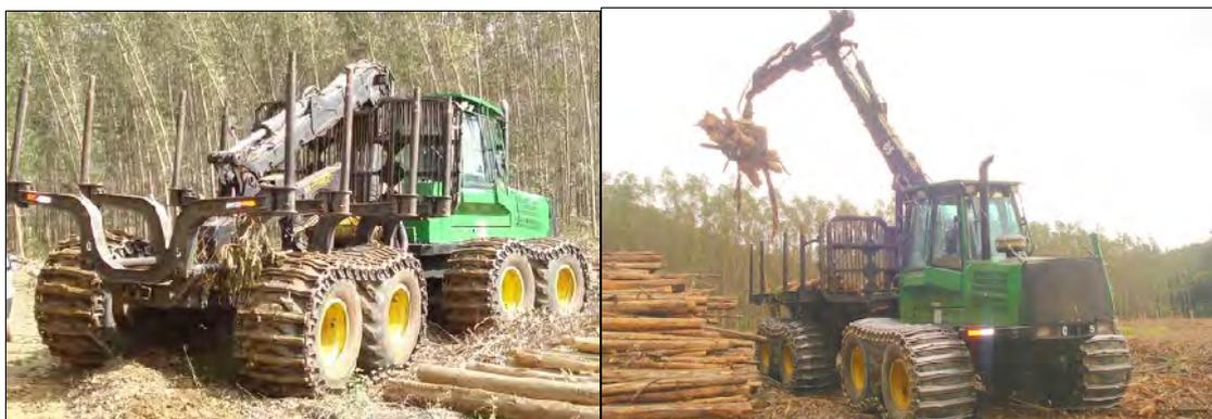
Figura 2.7 – Vista traseira e frontal do *Forwarder* John Deere modelo 1710D.
