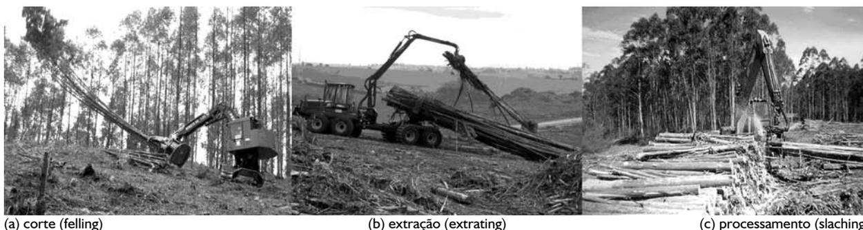
**Figura 2.** Máquinas utilizadas na colheita mecanizada no sistema tora longa, (a) "feller - buncher", (b) "clambunk" e (c) "garra traçadora". (Logging machinery used in the tree length system, (a) feller - buncher, (b) skidder and (c) slacher)
