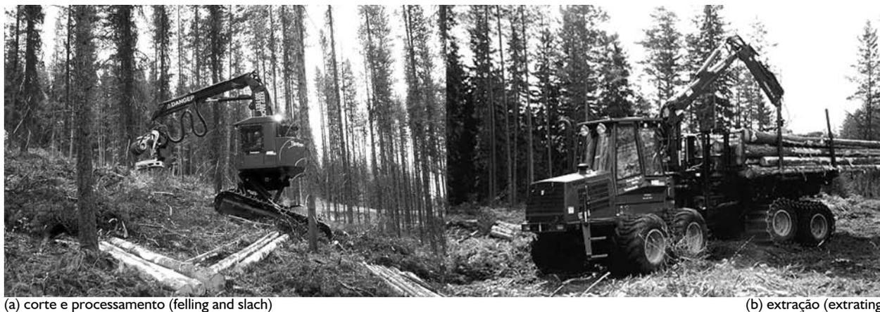
**Figura 1.** Máquinas utilizadas na colheita mecanizada no sistema tora curta, (a) "harvester" e (b) "forwarder". (Harvesting machinery in cut to length systems, (a) harvester and (b) forwarder)
