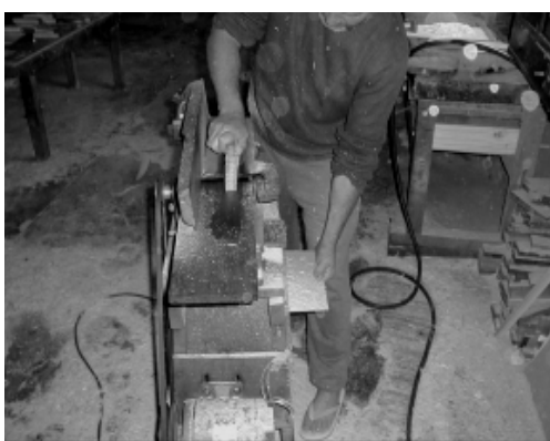
Figura 5. Processamento do disco na plaina. Figure 5. Processing the disc in the planer.
