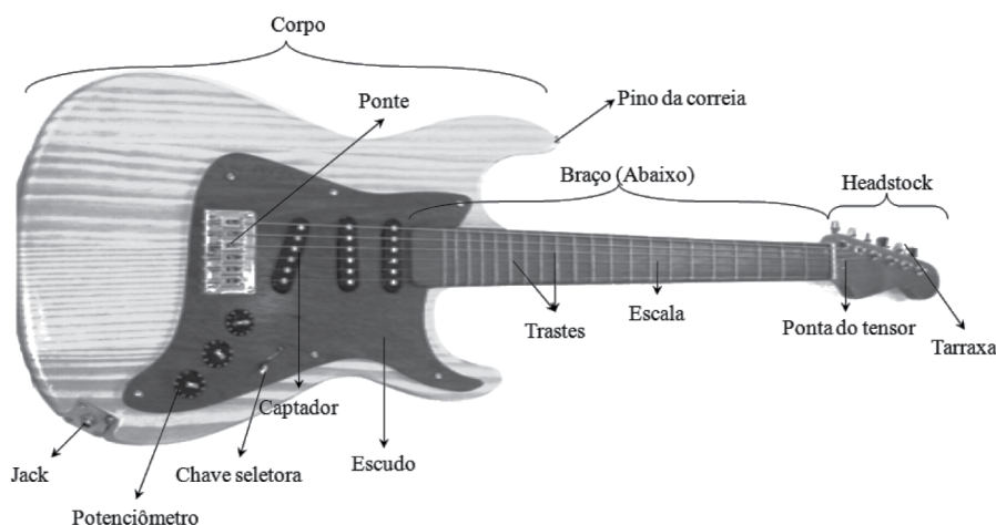
Figura 1. Componentes e partes da guitarra elétrica confeccionada. Figure 1. Components and parts of the electric guitar manufactured.
