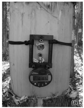
Figure 1. Determination of longitudinal residual strain (LRS): drilling of the stem (a), measurement of the strain through the extensometer (b).
