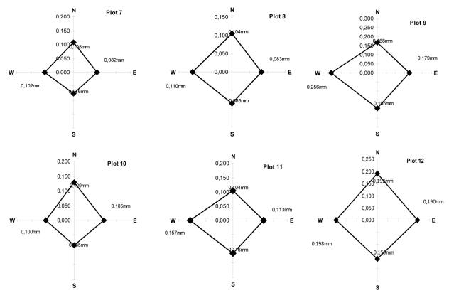
Figure 2 - Continuation. Distribution of longitudinal residual strain (LRS, in mm) in the four positions of readings around the stem of *Eucalyptus saligna* trees.
