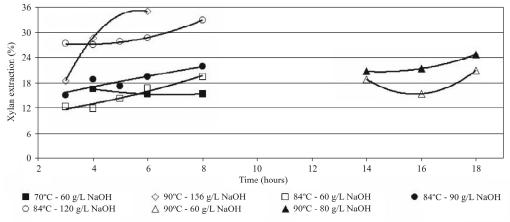
Figure 3 – Effect of NaOH concentration, reaction time and temperature on xylan extraction in the chips.
