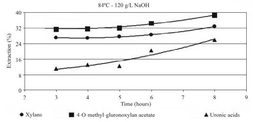
Figure 4 – Extraction of 4-O-methyl-gluronoxylan, acetyls, xylans and uronic acids at different intervals and with varying NaOH doses.
