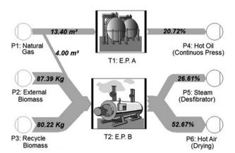
**FIGURE 3** Thermal Energy balance for 1.0 m<sup>3</sup> of MDF. **FIGURA 3** Balanço de Energia Térmica para 1,0 m<sup>3</sup> do MDF.
