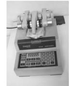
Figure 2. The *Taber Abraser* equipment used in the wear resistance test.
