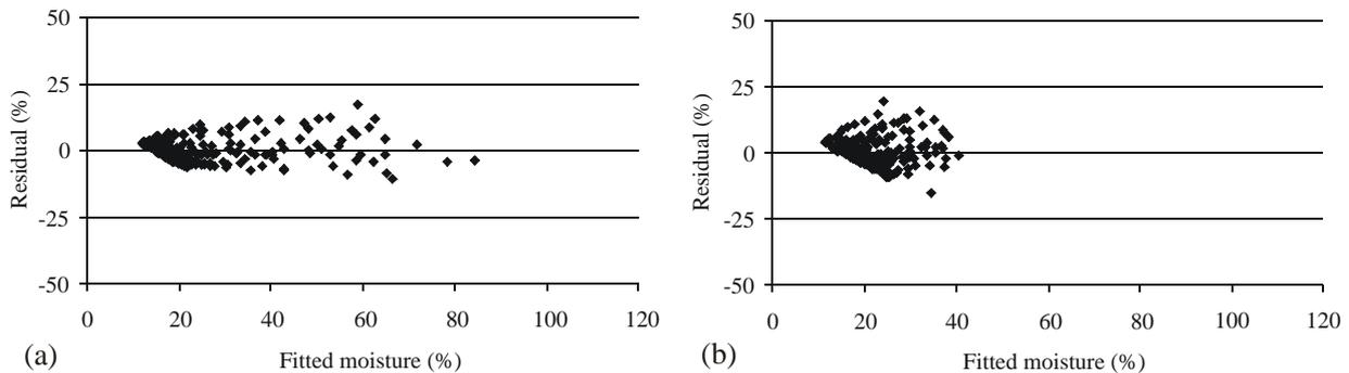
**Figure 4** – Scatter plot of fit residuals of the nonlinear equation estimating moisture content based on stress wave propagation in wood of *Eucalyptus urophylla* (a) and *E. cloeziana* (b).
