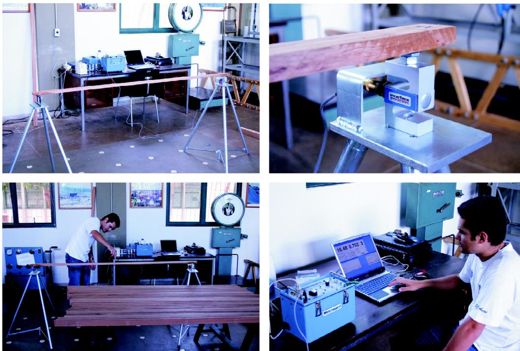
**Figure 1** – Nondestructive testing by transverse vibration.
