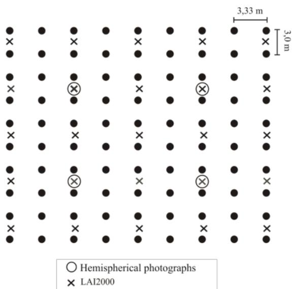
FIGURE 3: Sampling scheme performed by means of the LAI-2000 sensor and hemispherical cameras in the lines and between lines of the *Eucalyptus* stand.
